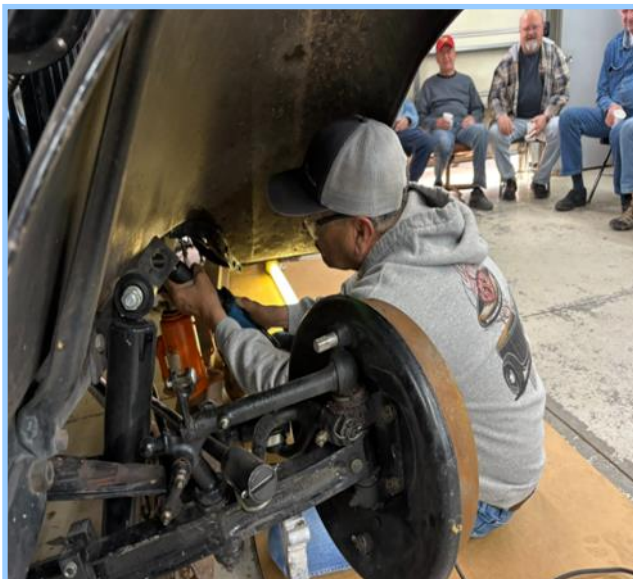
Figure 3 Jorge Preparing surface to weld. Observers in background.
