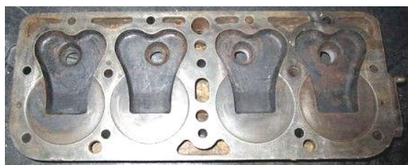
Unique combustion chambers, patented by Ricardo. 6 to 1 ratio.
