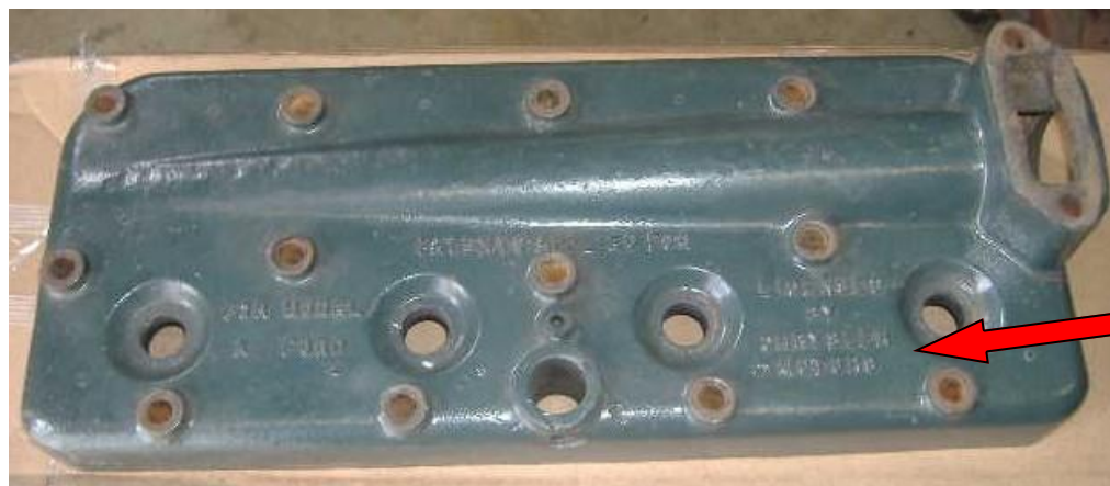
Head purchased on ebay. Note recessed spark plug holes.
