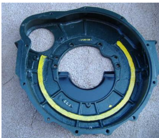
Late production housing with extended reinforcement.
