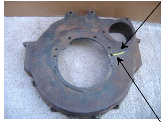
Original housing cracked on the driver's side.
