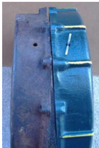
Original housing compared to late production housing with external reinforcement ribs. This feature can be checked by looking under the vehicle.
