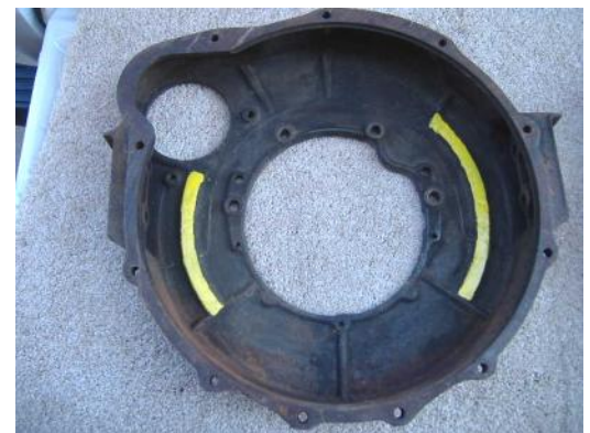
Inside original housing shows minimal reinforcement.
