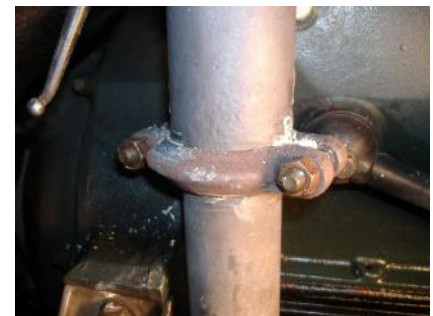
Excess sealant can be wiped off with your finger.
