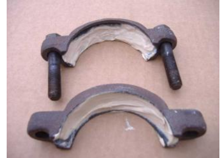
After wire brushing, apply sealer to both halves.
